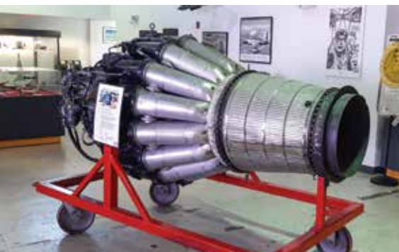
Photos this page clockwise from top left: Replica of the Wright Brothers first attempt at aviation; The Trautmann "RoadAir" flying car; Douglas A-4 Skyhawk; Allison J33-A-23 engine.
