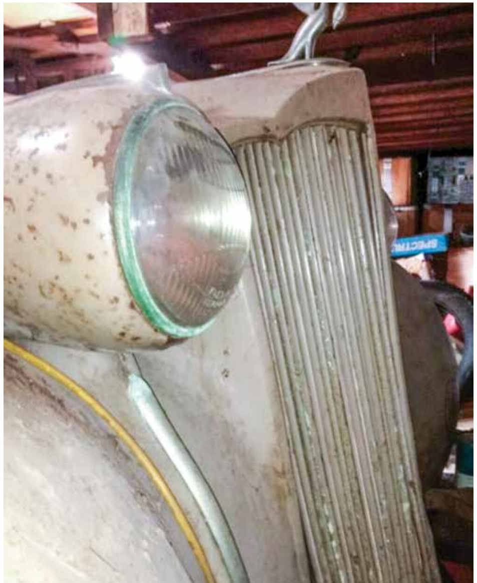
Eagle-eyed observers will notice two interesting features found on the eBay Packard. Notice the grille appears to have chromed shutters rather than the alternating chrome and black shutters usually found on 1939 Packard Twelves.
