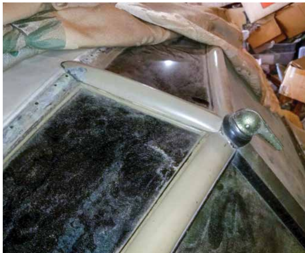
Brunn's signature Neutralite skylights above the windshield
